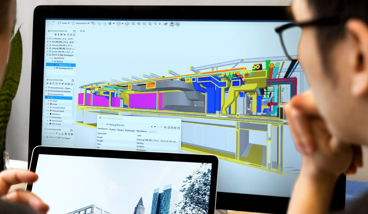
Virtual 3D collision testing. On the screen: the Brick technology story. © Schmidt Ploecker Architects
