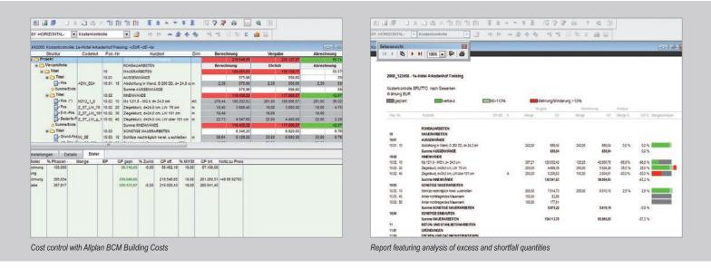
With Allplan Building Costs, you can reliably plan and track costs in connection with your TAI system. The package covers the whole area of tendering, awarding and invoicing contracts (for Allplan TAI). In addition, using the element data sheet, you can calculate costs according to the element method or create a room and building data sheet. Cost plans can be evaluated using various analyses according to service areas or the award structure.
