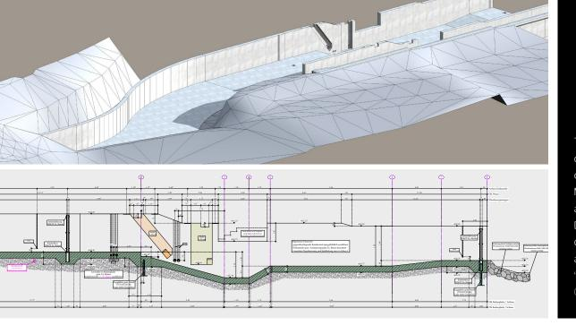
There are only a few offices that can accurately calculate a standing wave. McLaughlin Whitewater and Ben Nilsen from Denver/Colorado worked out the hydraulic design and the dimensioning of "The Riverwave". © concon
