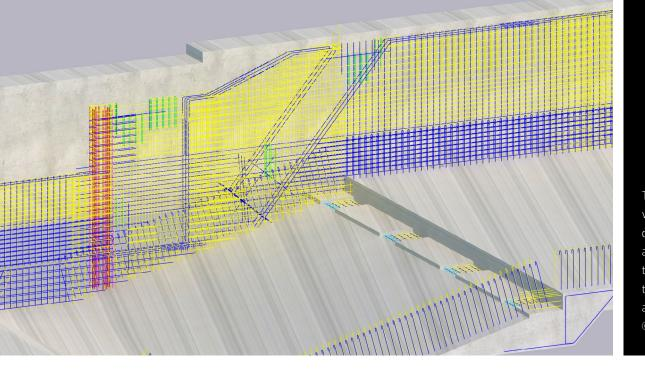
The entire reinforcement was designed threedimensionally in Allplan to avoid collisions between the complex intersections and wall recesses in advance. © concon
