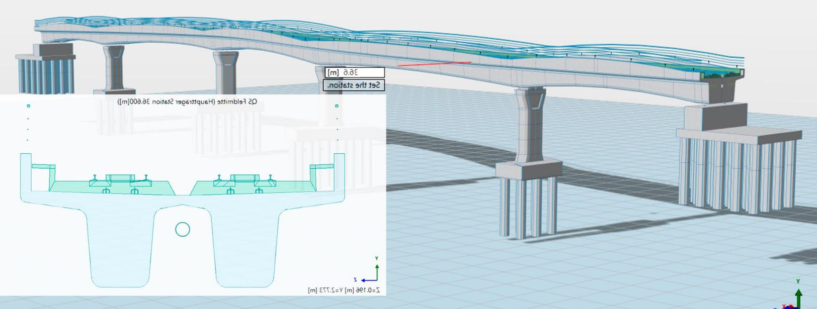
In Allplan Bridge 2021 it is possible to interactively displaying the cross-section at any point along the structure
