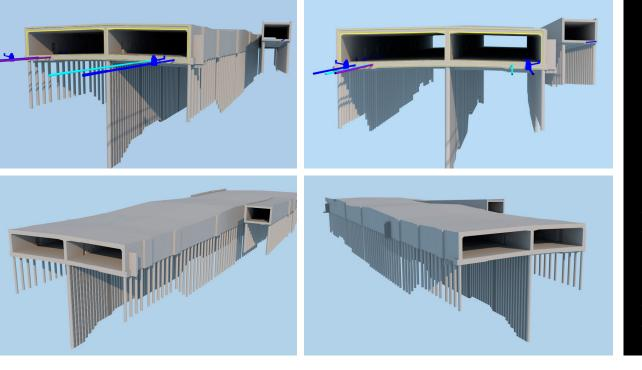
The high groundwater table in the area between the Elbe Tunnel and the S-Bahn Bridge necessitates a closed tunnel with combined pile slab foundations. © HOCHTIEF Engineering
