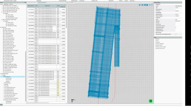
In Allplan Bridge, parametrically designed cross-sections can be created georeferenced along an axis. HOCHTIEF Engineering used this for fast and precise planning of the tunnel with all variations and details. © HOCHTIEF Engineering
