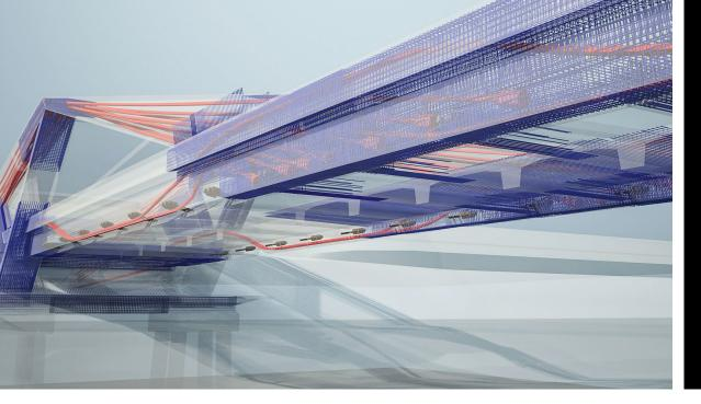
", Thanks to the visualization in the 3D model, we were able to prove the feasibility of the dimensions for the knot we selected with reinforcement and pre-tensioning."
